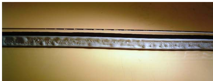
Figure 4: QUV Exposure Samples - 1,283 exposure hours
